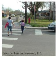
This 24-inch stop line has been correctly installed at least 4 feet in advance of the marked crosswalk.
