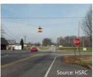
This oversized STOP sign is supplemented by an Intersection Control Beacon.
