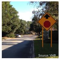
This oversized Advance Traffic Control sign requires two supports, which have been supplemented with reflective panels.
