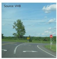
The lane assignment pavement markings at this T-intersection help notify the road user of the impending intersection.
