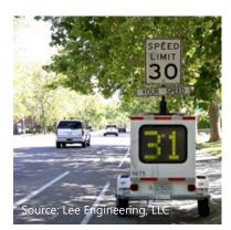
The Speed Limit sign and dynamic feedback sign assembly can be moved from location to location using a mobile trailer such as this.
