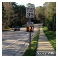
A dynamic feedback sign displays the speed of an approaching vehicle.
