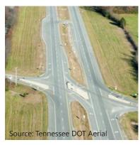
This aerial photograph shows the channelization at the intersection and the downstream U-turn bulb-out.
