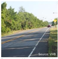
Transverse rumble strips are installed ahead of this yield-controlled intersection.
