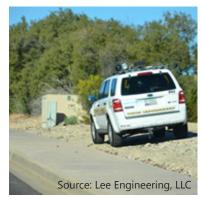
This SUV is deployed for automated speed enforcement through photos.
