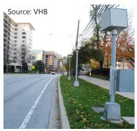
These speed enforcement cameras are positioned in advance of a pedestrian crossing of the uncontrolled major road at the unsignalized intersection ahead.
