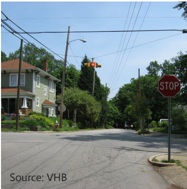
Source: VHB The Intersection Control Beacon flashes red from the stop-controlled approach.
