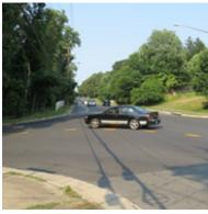
These dotted turn path markings are yellow because they guide left-turning drivers from the major road double yellow center line to the minor road double center line.
