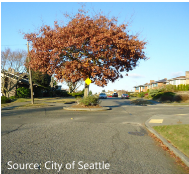
Source: Lee Engineering, LLC The large, landscaped center island provides a traffic calming effect along this wide and straight residential street.
